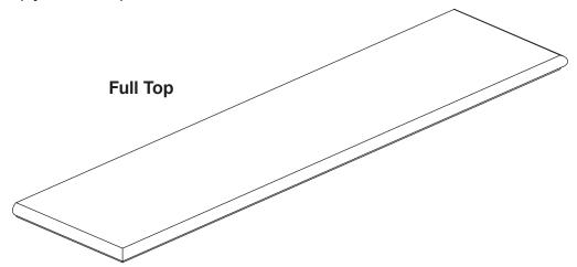
Alternatively, you may simply have a Top 'lip'. This can be located using Dowels, and glued or screwed from above. This may be supplied as one single component or several parts which join together with a Connector (using the hex key provided) once in place.
