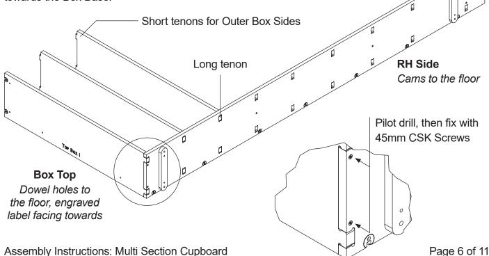
9. Once the Shelves and the Box Base assembly are placed in the RH Side, the LH Side can be located. Ensure that the Shelves with cams align with the Cam Bolts in the LH Side, and lock these into place. Lock the cams in the Box Top and Box Base.
