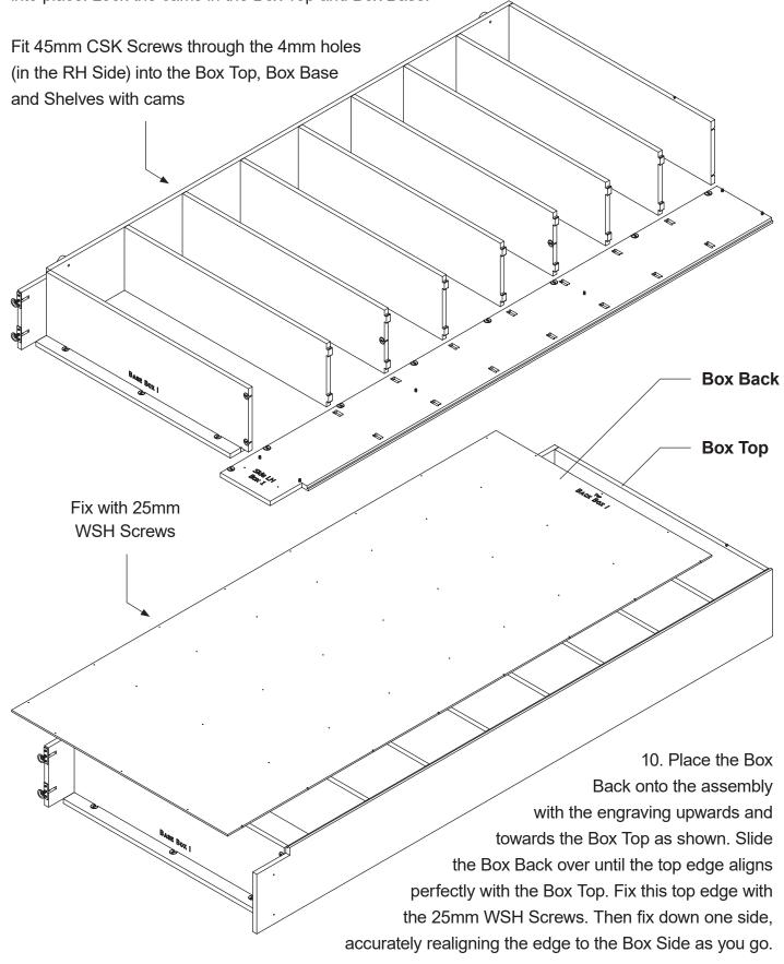
This should force the box square. Once all sides are fixed in place, continue to screw through the remaining 3mm holes with 25mm WSH Screws to help secure the Shelves.
