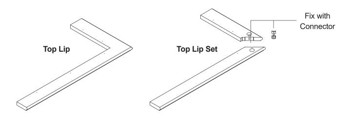
Locate the Top to the Box Tops using Dowels. It can be glued into place, screwed into place from beneath, or left as is. For 30mm Tops, use 45mm CSK Screws. For 18mm Tops, use 30mm CSK Screws. For exceptionally wide units, the Top and Skirting may be supplied in several lengths.
