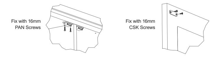
17. Fix Magnetic Catches to the required Box Tops with 16mm PAN Screws. The Catch should be towards the front, with the magnet facing outwards. Then, fix Magnetic Catch Plates to the back of any Doors with 16mm CSK Screws.
