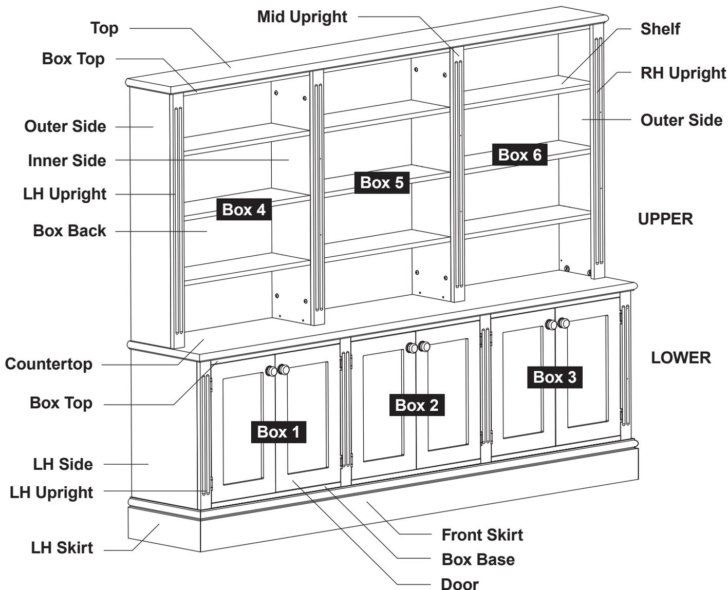
Here's just the example lower section in more detail. Each box is made up of a Box Top, Box Base, Box Back, LH Side, RH Side and Valance. Look out for engravings to help identify parts. Depending on your design, boxes may feature Shelves, Dividers and/or Doors. Refer to the Parts Diagram to confirm this arrangement.
