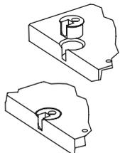
2. Push the Cam, facing outwards, into the corresponding hole on the other part.
