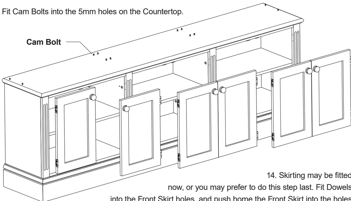
14. Skirting may be fitted now, or you may prefer to do this step last. Fit Dowels into the Front Skirt holes, and push home the Front Skirt into the holes on the Uprights and Valances. This can be glued into place, or left as is.
