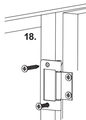
18. Fix Doors in place with Hinges and 25mm CSK Screws. Ensure the butt of the hinge clears the edge of the door, so the doors are positioned correctly.
