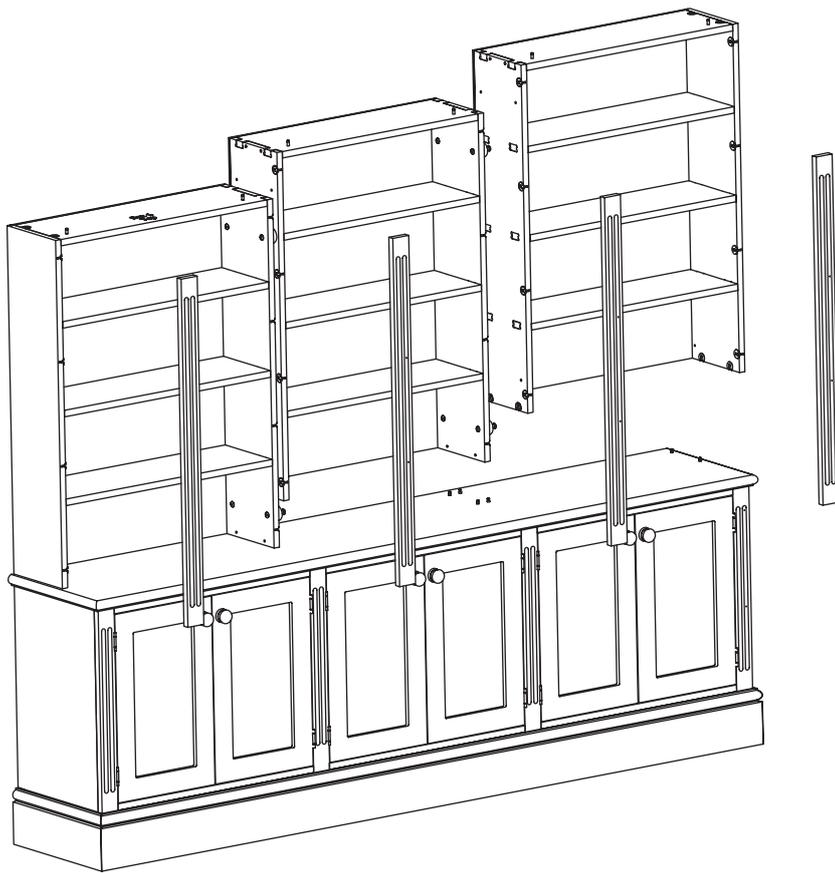
20. The upper section boxes fit onto the Countertop by aligning and locking the Box Side cams with the Countertop Cam Bolts.
