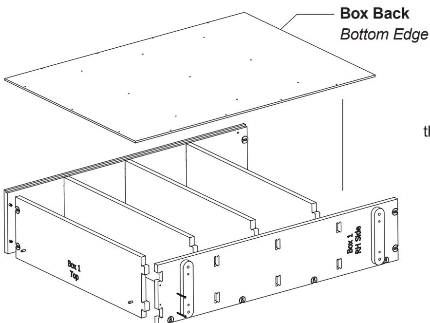
The Back must be flush with the bottom of the two Sides to ensure that it sits neatly on the Countertop.
