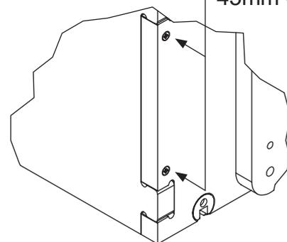
8. Once the Shelves and the Box Base are placed in the RH Side, the LH Side can be located. Ensure that the Shelves with cams align with the Cam Bolts in the LH Side, and lock these into place. See Page 2 for help with cams. Lock the cams in the Box Top and Box Base.
