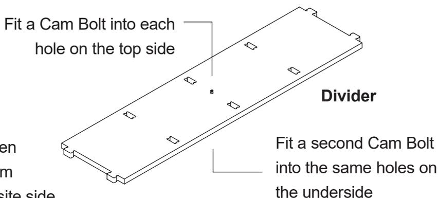
4. On taller units, one or more of the outer Shelves (in the outer boxes) may have a cam hole. Place Nickel Cams in these.
