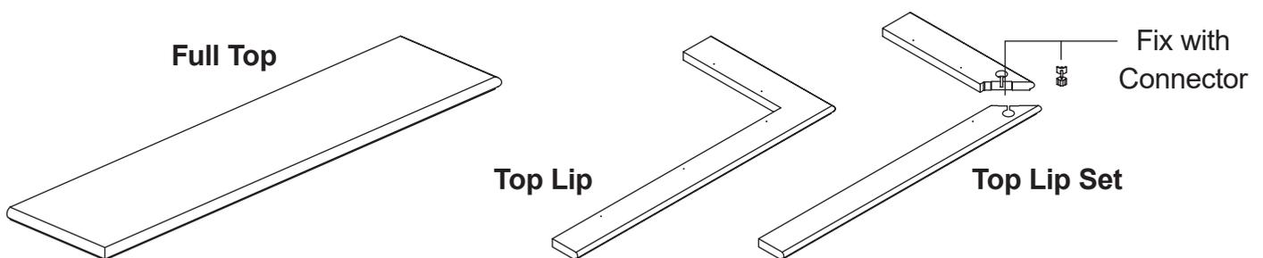
Alternatively, you may have a Top 'lip'. Attach this in the same way. This may be supplied as one single component or several parts which join together with a Connector (using the hex key provided) once in place.
