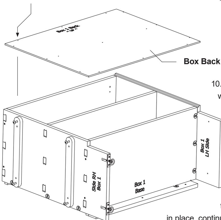
10. Place the Box Back onto the assembly with the engraving upwards and towards the Box Top as shown. Slide the Box Back over until the top edge aligns perfectly with the Box Top. Fix this top edge with the 25mm WSH Screws. Then fix down one side, accurately realigning the edge to the Side as you go. This should force the box square. Once all sides are fixed in place, continue to screw through the remaining 3mm holes with 25mm WSH Screws to help secure the Shelves.
