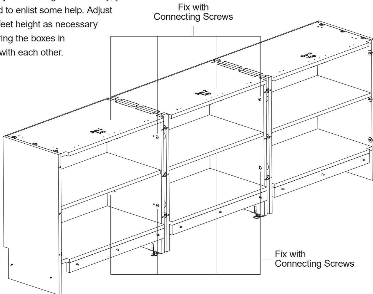
To lock the Mid Upright cams, use a pozi screwdriver via the access holes on the Inner Box Sides
