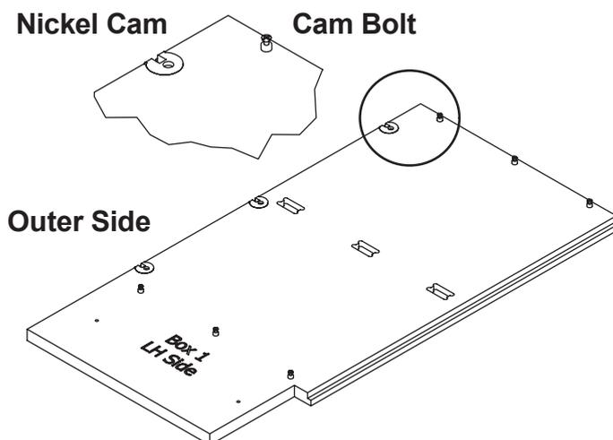
2. For all the remaining Box Sides use White Cams instead, as they will be hidden. Place the White Cams in all the available holes, facing outwards. Attach the Adjustable Feet using the Foot Plate and 20mm PAN Screws for each assembly. However, you should pilot drill these first to avoid splitting the wood. The Adjustable Foot should be set to about 25mm.
