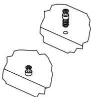
1. Screw in the Cam Bolt, up to the shoulder, into the 5mm hole in one part.
