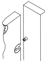
3. Push the two parts together, so that the Cam Bolts disappear into the middle of the Cams.
