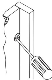
4. Insert a 5mm Pozi screwdriver – tilt back at a slight angle – and rotate CW to lock the Cam.
