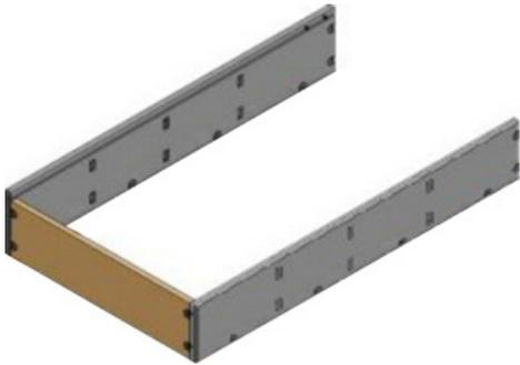
Place White Cams in the Box Top. The Box Top can be placed between the two Sides, with its two 6mm holes facing the front of the finished section (towards the floor), and the White Cams facing outwards.
